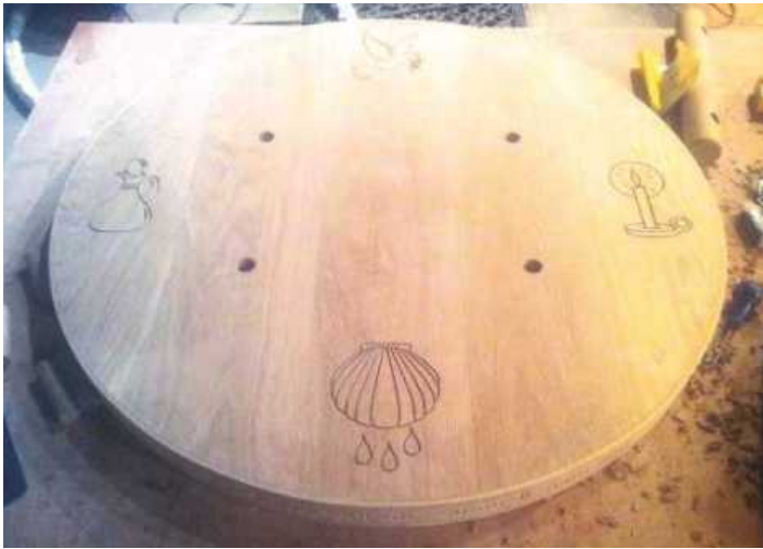
▲ Pic.21 Holes were drilled in the font cover and bottom of the handles using a 20mm auger bit
